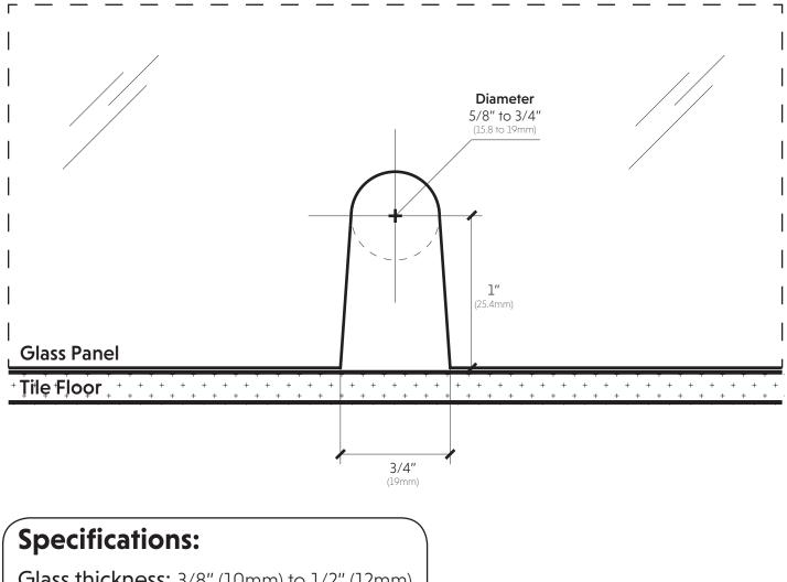
Glass thickness: 3/8" (10mm) to 1/2" (12mm) tempered glass only. Construction: solid brass (cutout required) Includes: gaskets, screws and fabrication dimensions
