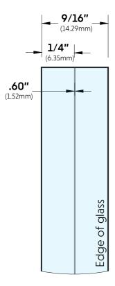
Material: Two tempered glass panels bonded together with a PVB interlayer
