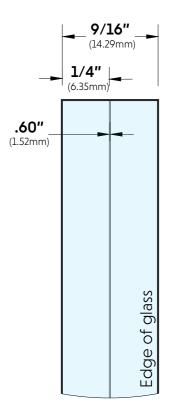
Material: Two tempered glass panels bonded together with a PVB interlayer
